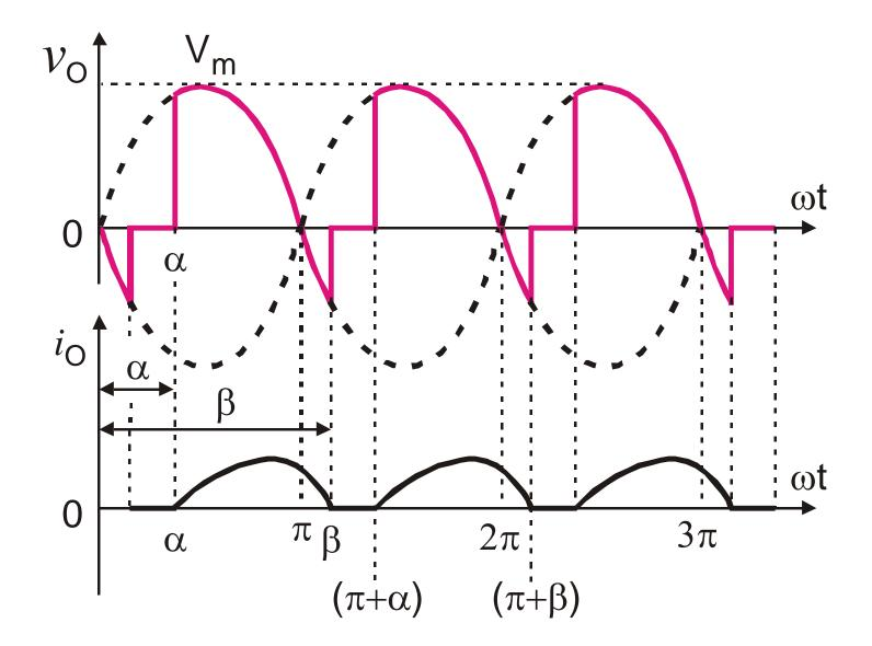
$$V_{O(dc)} = V_{dc} = \frac{1}{\pi} \int_{\omega t = \alpha}^{\beta} v_{O}.d(\omega t)$$
