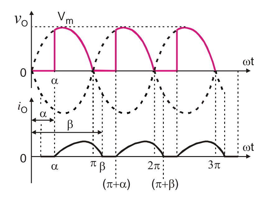
Thyristor  $T_1$  is triggered at  $\omega t = \alpha$ ;  $T_1$  conducts from  $\omega t = \alpha$  to  $\pi$ Thyristor  $T_2$  is triggered at  $\omega t = (\pi + \alpha)$ ;  $T_2$  conducts from  $\omega t = (\pi + \alpha)$  to  $2\pi$ FWD conducts from  $\omega t = \pi$  to  $\beta$  &  $v_o \approx 0$  during discontinuous load current.
